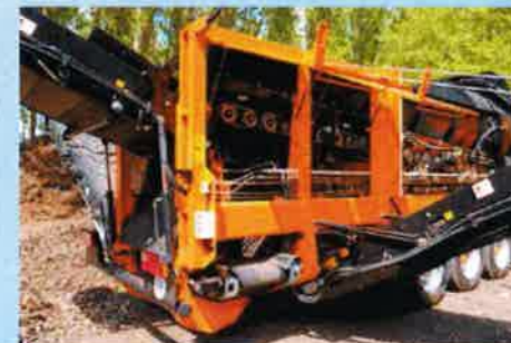
Large side doors for maintenance
